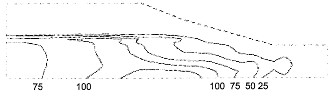
Fig. 12. Undrained response under placement of fill material: (a) Displacement vectors, (b) Contours of excess pore pressure
