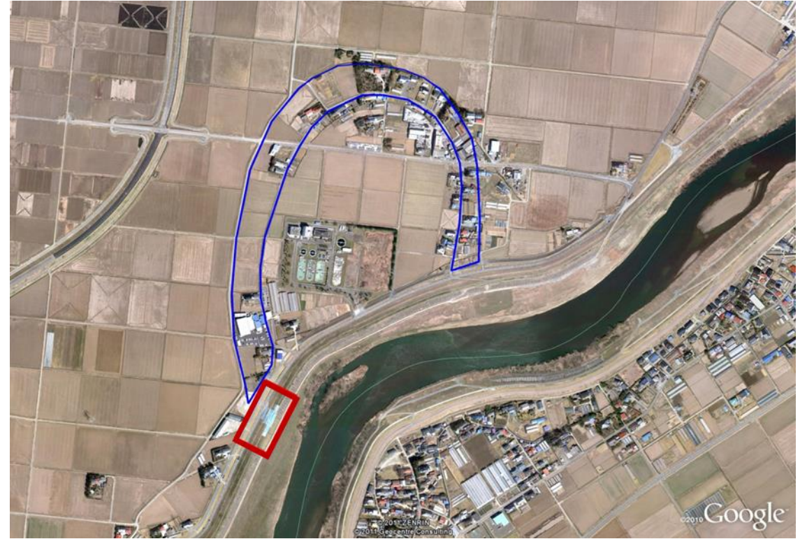
Levee damages coinciding with a mapped paleochannel (MLIT 2011, GEER 2011)
